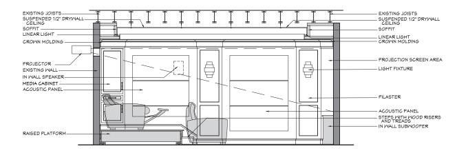
**BUILDER'S NOTE:** The owner mentioned possibly incorporating tiered seating in the theater. Luckily the existing ceiling was dropped and could be raised up so the higher seats would not feel cramped. A perimeter soffit was added for uplighting to enhance the ambiance. The entrance doors were moved closer to the screen to give more room for the seating area and provide symmetry for the new pilasters. The pilasters serve multiple functions including providing a traditional element to
